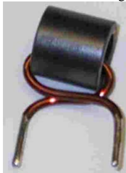
Figure 6: 1 turn ferrite bead for snubber inductor
