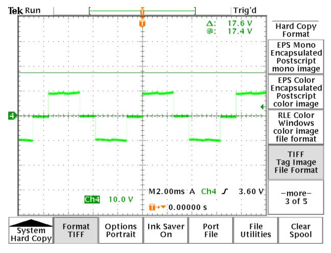
Figure 1: Typical Voltage Waveform, measured with differential probe
