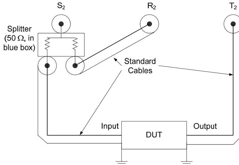
Notice that the input and output must be ground-referenced. The  $T_2$  terminal can tolerate a few volts of dc offset, but it is still a good idea to capacitively couple both connections (e.g.  $2.2 \mu\text{F}$  monolithic). A splitter has been built in a small blue aluminum box.
