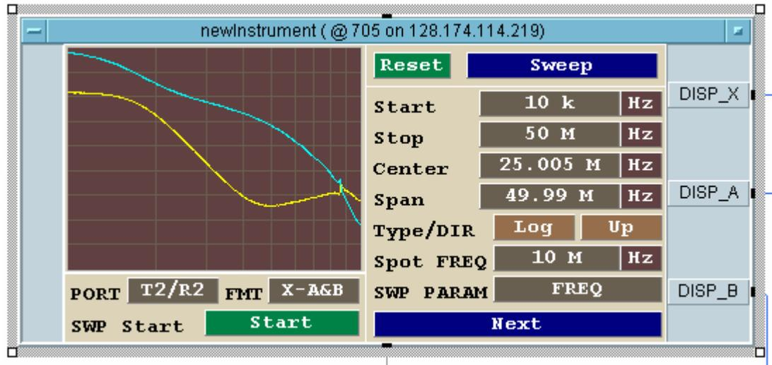
Click on the Start frequency and enter the new start. Click on the Stop frequency and enter the new stop. So in the image above, the range has been set to 10 kHz – 50 MHz. Click on the “Type” until it again says “Log.”
