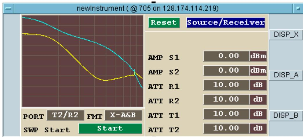
Some errors result from not following the setup procedure properly or the instrument somehow getting in a strange mode. Just because the VEE panel looks right, the HP4195A might not be in the right mode. For example, VEE might say the sweep is in LOG mode, but the HP4195A might be in linear. Toggle a couple times to make sure the instrument is actually in LOG mode.
