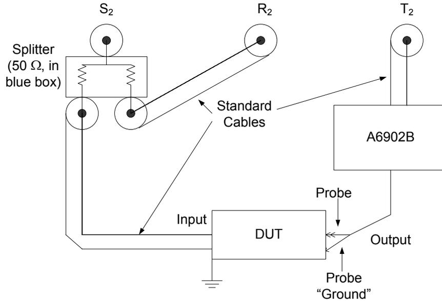
Typically, set the A6902B on ac coupling and 100 mV/div (1X). This method is effective for low-voltage systems.
